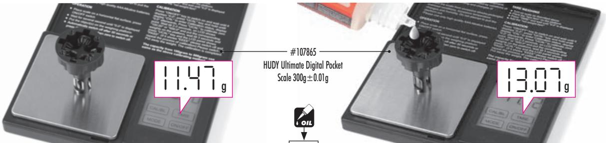
1 Put the diff (without oil) on the scale and check the weight (approximately 11.47g)
