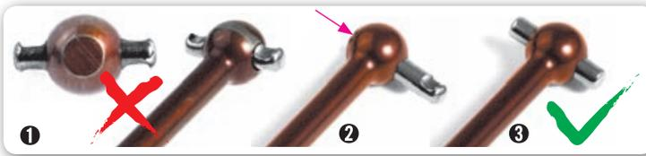
**DO NOT** use drive shafts when the pins are worn.
