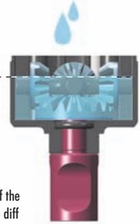
Fill differential up to the top of the diff cross-pins. DO NOT fill the diff to the top of the housing.
