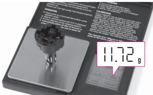
1 Put the diff (without oil) on the scale and check the weight (approximately 11.72g)
